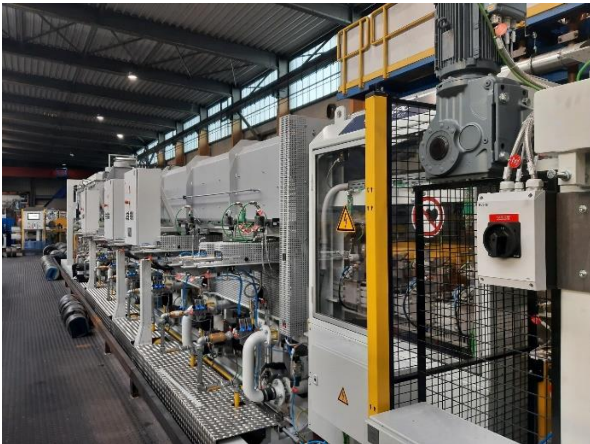
Billet oven and preheating system by extrutech in use at apt: Sustainability, quality, and efficiency as priorities in the energy-optimized heating process
